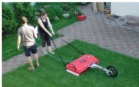
Deployment of GPR with various antennas
