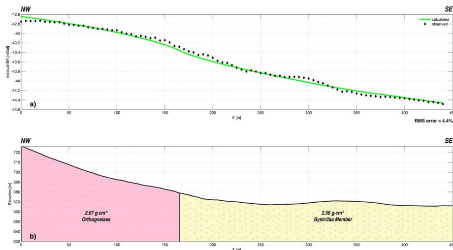
**Fig. 8.** Density modelling results. (a) Observed (black diamonds) and calculated (green line) gravity anomalies related to the constructed density model (b).
