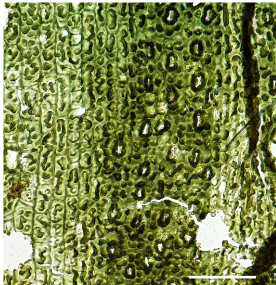
Figure 2. Abaxial cuticle of new cordaitalean cuticular morphotype with a stomatiferous band and papillose cells. Upper bench of the Kounov coal seam, Hokov-Děkov locality, scale bar = 100 \mu m.
