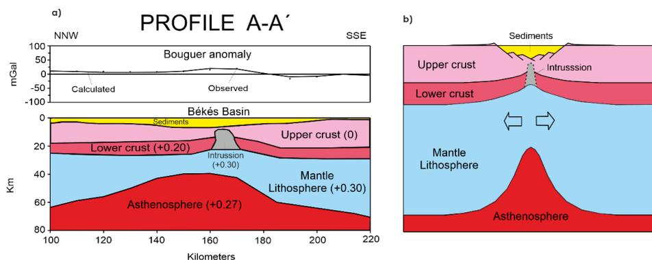
**Fig. 23.** (a) Density model along the profile A-A'. The density contrast values are in  $g\ cm^{-3}$ . (b) Scheme of a narrow rift model (sub-basin) of continental extensional tectonics for the Pannonian Basin System (modified after Bielik & Ádám 2006).
