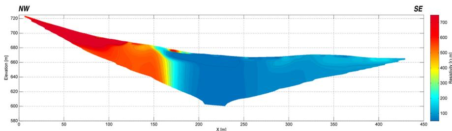
**Fig. 7.** Resistivity cross-section along the Profile A-A' constructed from electrical resistivity tomography measurement.
