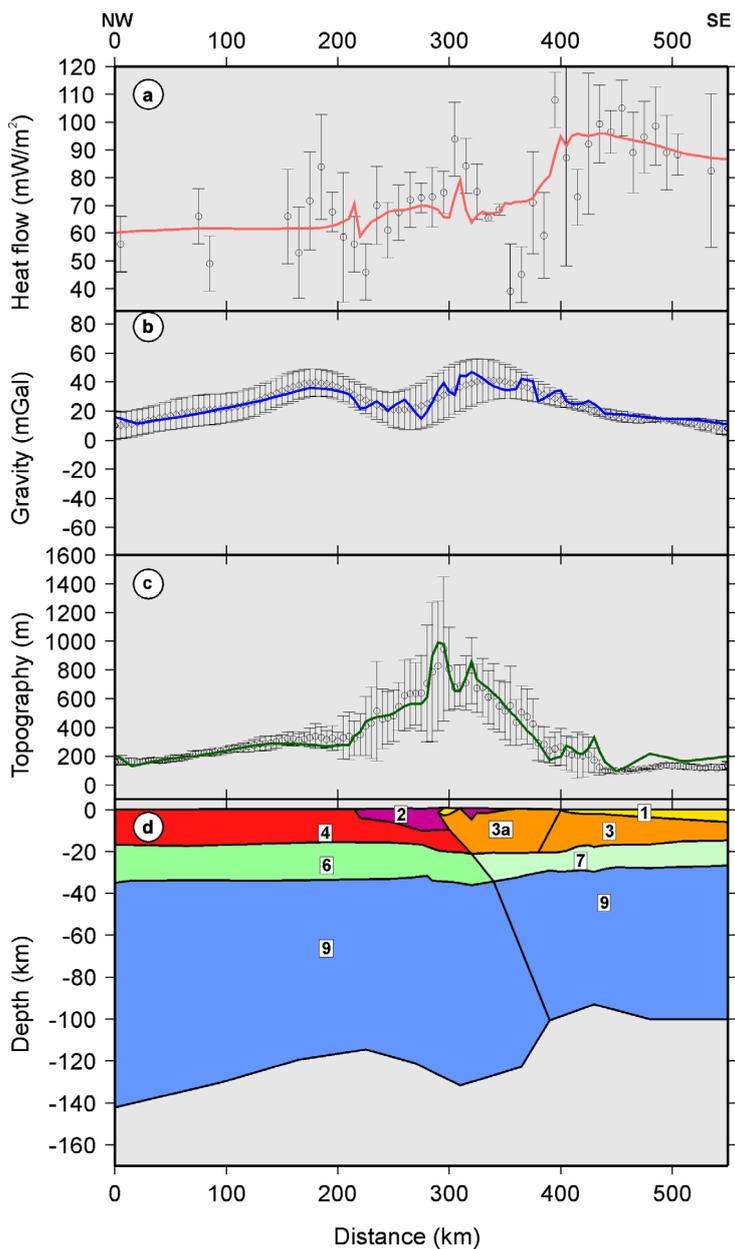
**Fig. 15.** Lithospheric model along transect IV. (a) Surface heat flow, (b) free air gravity anomaly, (c) topography with dots corresponding to measured data with uncertainty bars and solid lines to calculated values. Numbers in (d) correspond to material number in Table 2 (Zeyen et al., 2002).
