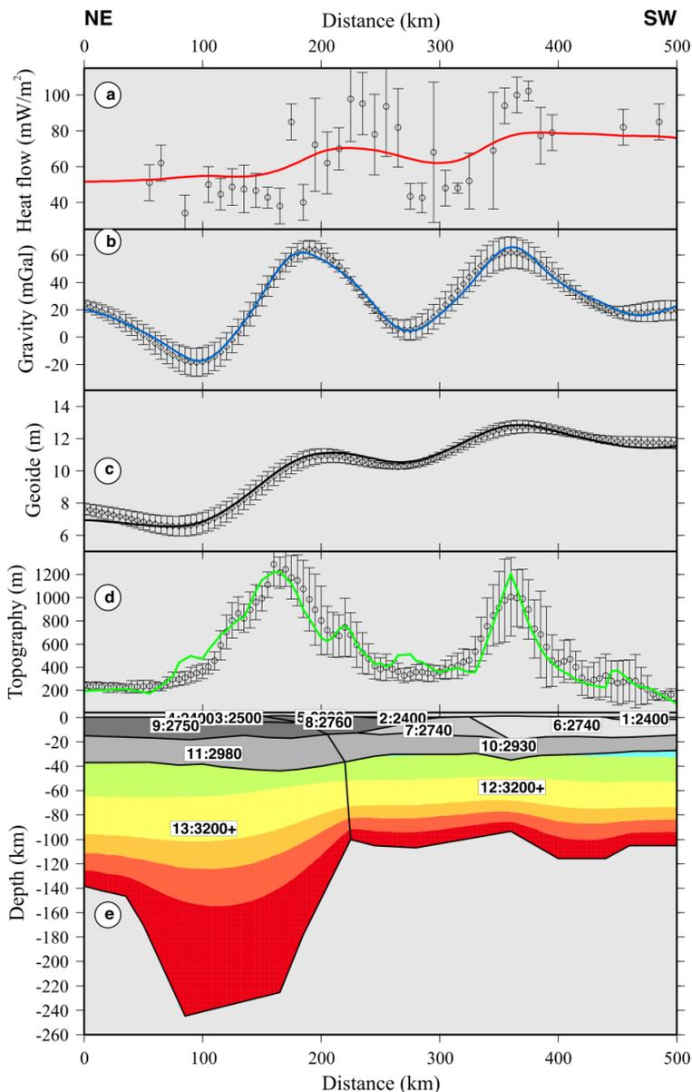
**Fig. 16.** Lithospheric model along profile VII. (a) Surface heat flow, (b) free air gravity anomaly, (c) topography with dots corresponding to measured data with uncertainty bars and solid lines to calculated values. Numbers in (d) correspond to material number in Table 3 (Dérerová et al., 2006).
