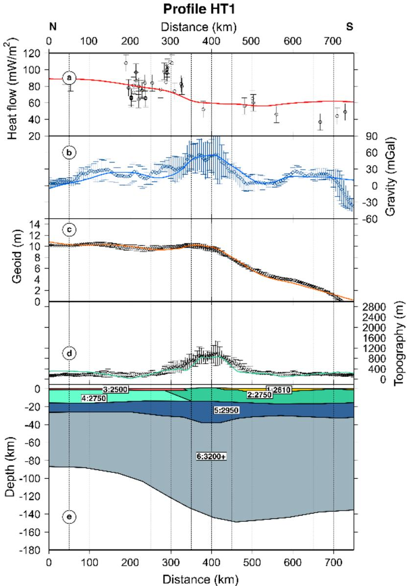
**Fig. 20.** Lithospheric model along transect HT-1. (a) Surface heat flow, (b) free air gravity anomaly, (c) geoid, (d) topography with dots corresponding to measured data with uncertainty bars and solid lines to calculated values. Numbers in (e) correspond to material number in Table 4.
