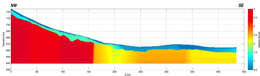
**Fig.6.** *P-wave velocity cross-section along the Profile A-A' constructed from seismic tomography measurement.*
