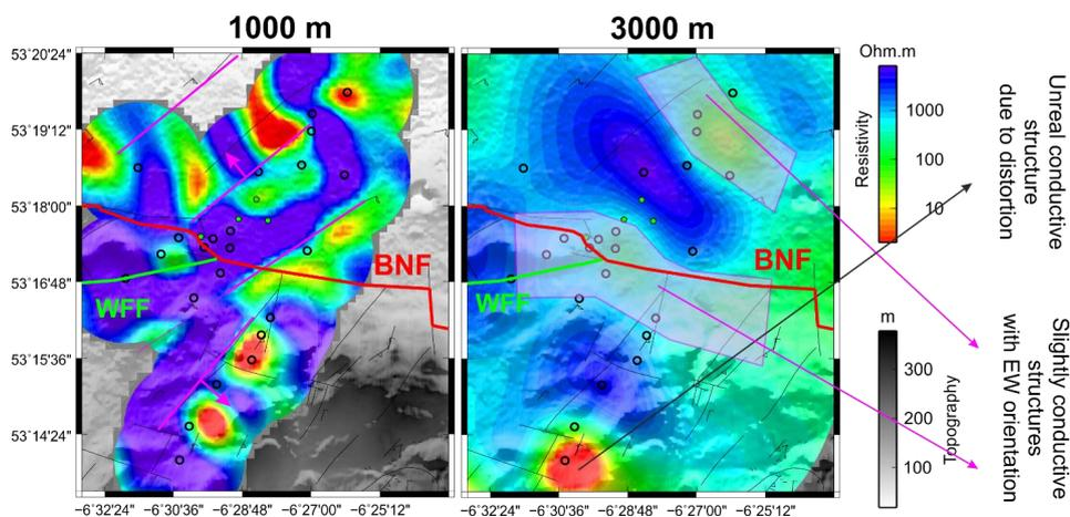
Fig. 3: Horizontal sections at depth 1km and 3km with indicated main features in the model and its possible interpretation. The purple lines in 1km section highlight strong lateral boundaries which are correlated with surface traces of faults (WFF - Wheatfield Fault). The 3km section show deeper conductive structures, which are oriented along the BNF (purple semi-transparent areas). The high conductive structure in the south is interpreted as unreal structure (black arrow).
