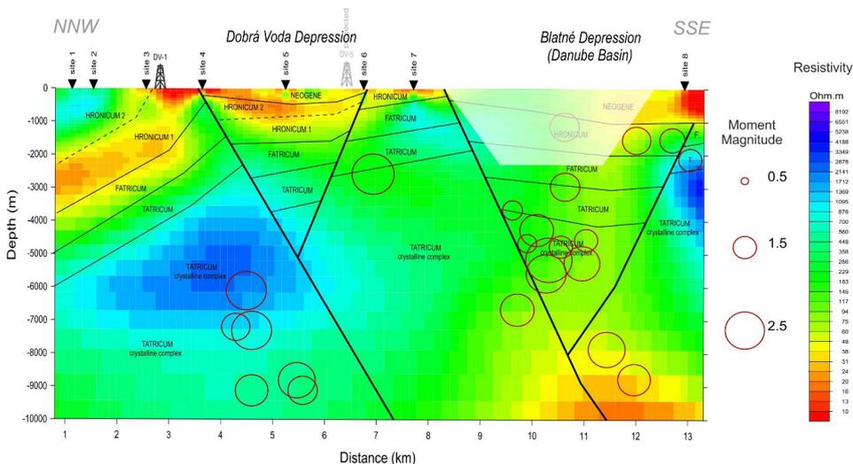
Fig. 4: The final 2D model of the MT profile DVMT01 with interpreted tectonic structures and positions of earthquake hypocentres. Shaded area indicates low resolution part of the model.
