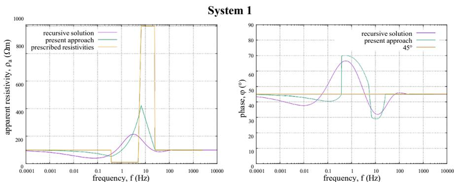
**Figure 5.** Computed apparent resistivity and phase difference between electric and magnetic fields for Half-space 1. The dependences obtained as a result of this study show sharp changes that reflect sharp transitions in the physical conditions at the interfaces between the layers.
