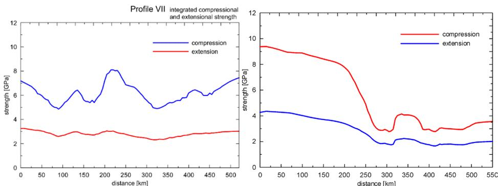
**Fig. 17.** Vertically integrated compressional (blue line) and extensional (red line) strength calculated along profile VII (left) and IV (right).
