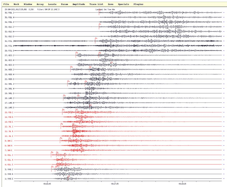
**Fig. 3.** An example of a manual local event interpretation using the Seismic Handler package. Displayed traces are from the Virtual Regional Seismic Network in the ESI SAS Bratislava for the January 28, 2021,  $M_L=3.2$  local earthquake from the Vtáčnik Mts., Slovakia.
