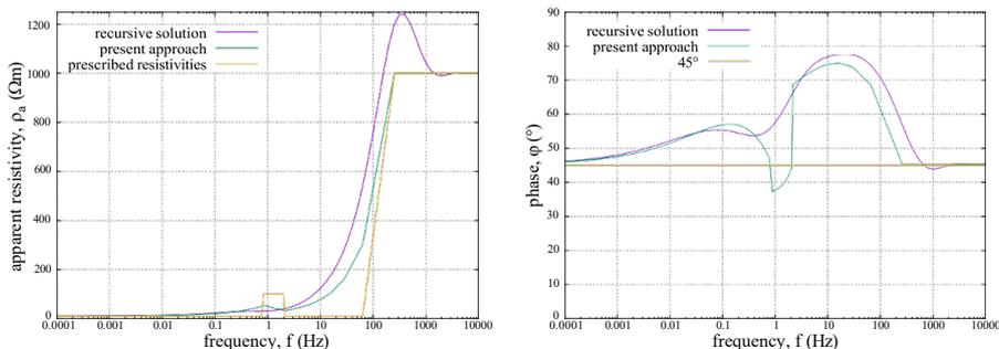
**Figure 6.** Computed apparent resistivity and phase difference between electric and magnetic fields for Half-space 2. The dependences obtained as a result of this study show sharp changes that reflect sharp transitions in the physical conditions at the interfaces between the layers.
