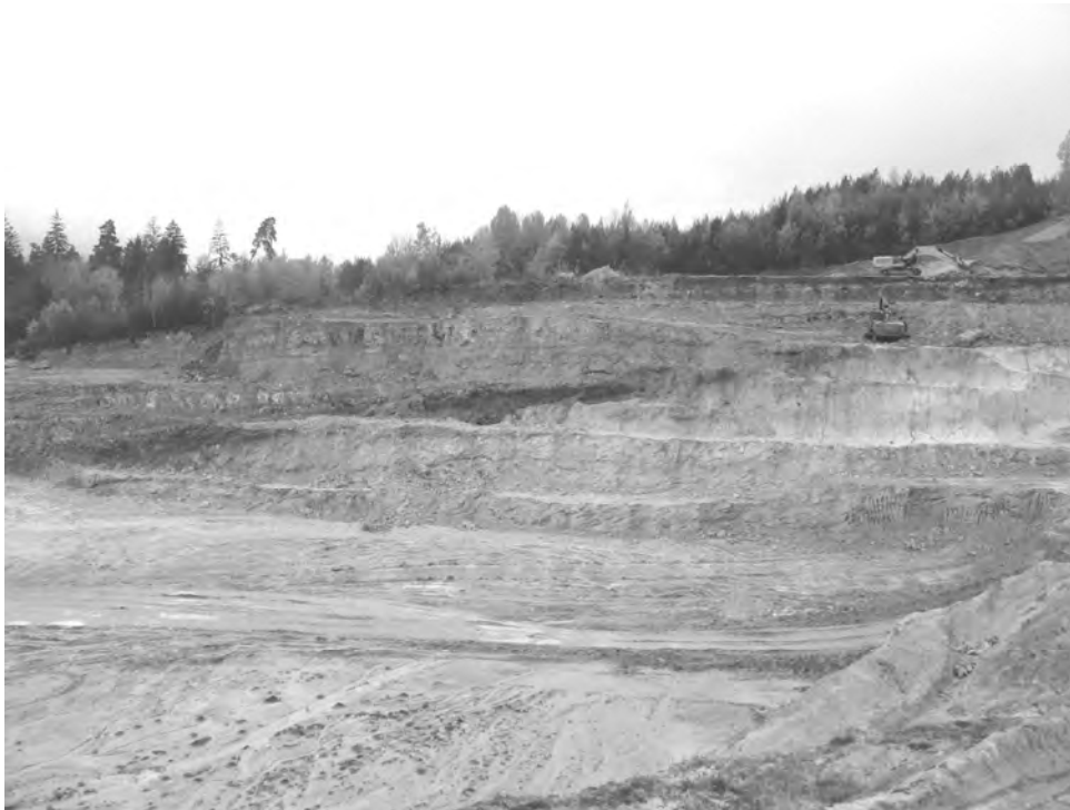
Fig. 15 Quarry Jelšový potok. Bentonite (light), object of exploitation, is covered by silica sinter sequence (dark).
